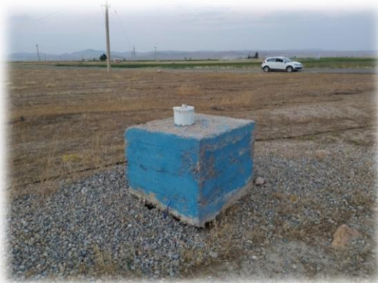
Fig. 6- Sefiddasht plain, southwest side of the plain UTM Coordinates= x: 513390 - y: 3550574 Subsidence: about 7 cm (02/08/2022)
