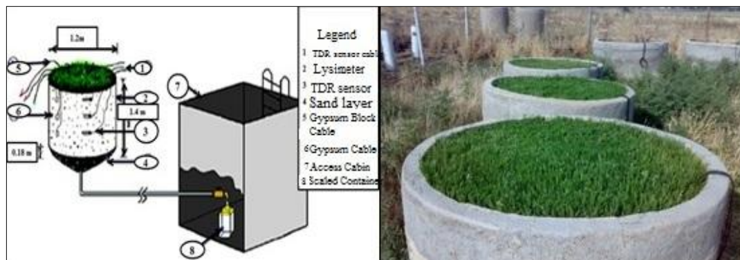
Fig. 2- Lysimeter cultivated with grass, Water drain chamber
