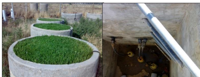
Fig. 2- Lysimeter cultivated with grass and water drain chamber
