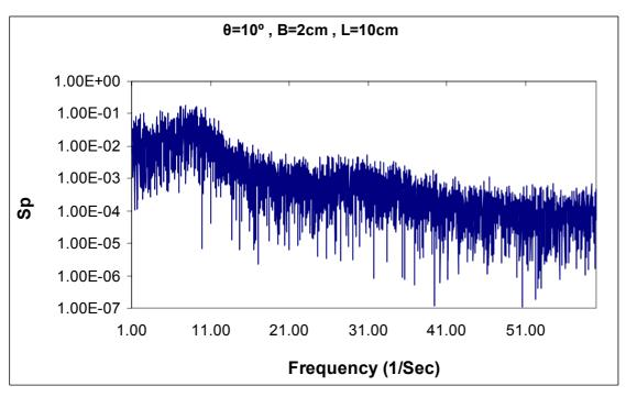
Figure 9- Frequency spectra of pressure fluctuations downstream of ramps.
