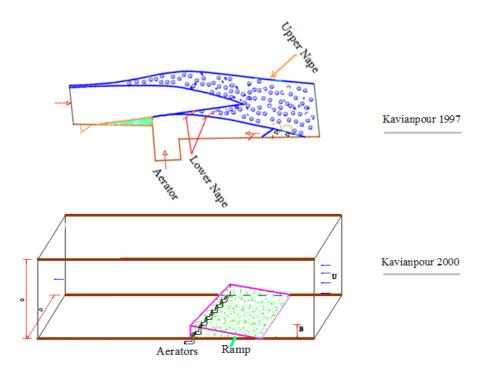
Figure 5- Schematic view of experimental studies (Kavianpour, 1997, 2000)
