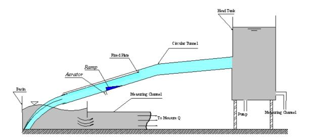
Figure 1- A schematic view of experimental setup.
