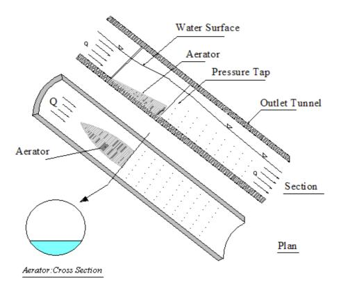
Figure 2- The arrangements of aerator and pressure taps.
