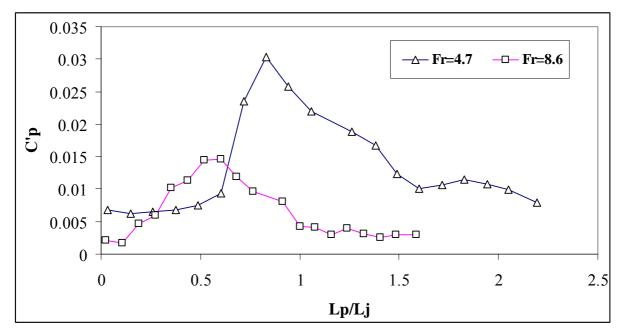
Figure 3- Variations of pressure fluctuations with Froude number on the centerline of the tunnel (B=1 cm).
