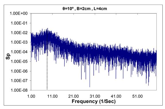
Figure 8- Frequency spectra of pressure fluctuations downstream of ramps.
