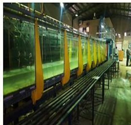
Fig. 4- Concentration measurement at 5 different sections in the downstream of the tracer injection
